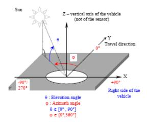
hemisphere described by the azimuth and elevation angles. Both parameters are specified in angular degrees – the azimuth from 0° to 360° and the elevation from 0° to 180°. The degrees of azimuth define the incoming solar radiation in the horizontal plane, where 0° designates the direction of travel. The degrees of elevation describe the incoming solar radiation in the vertical plane, where 90°C corresponds to solar rays coming directly from
