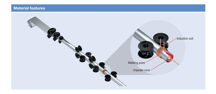
TDK has introduced IPH2 material, which has lower reluctance than the original IPH material at higher temperatures. IPH2 material is tuned to have lower loss closer to the application temperature. It has a slightly higher saturation flux density than the well-accepted IPH material currently in use in the industry.
