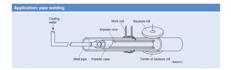
An impeder core is an essential accessory for welding tubes and pipes using high frequency waveguide heating. The impeder core concentrates the magnetic flux generated by the work coil into the area of the pipe joint. Consequently, using an impeder core greatly increases the efficiency of the welding process.
