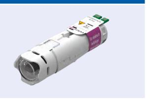
This module is designed for the surface treatment of non-conductive substrates such as plastics, ceramics or glass. For effective treatment, a module-substrate-distance of 1 to 5 mm is recommended. If uncontrolled arcing occurs on the substrate during use, the device switches off automatically. In this case the surface is at least partially conductive and should therefore be treated with the Module nearfield.
