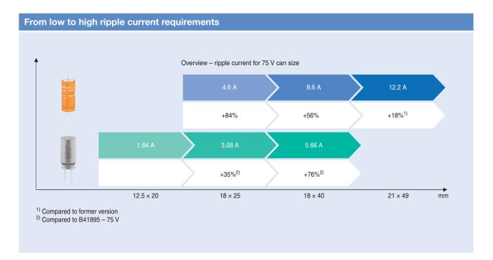
Axial-lead capacitors offer advantages over standard single-ended designs when very high ripple current is requested. Special design technologies enable a significant reduction of the Equivalent Series Resistance (ESR) of the capacitors and therefore higher ripple current capability.
