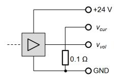
Fig. 2. Output stage of the CeraPlas driving circuit
