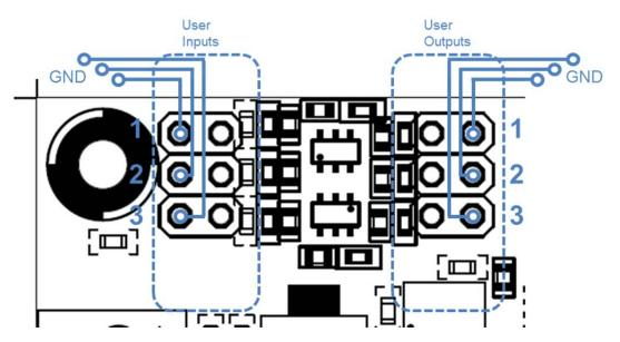
Fig. 2. CeraPlas driving circuit definition of the user IO
