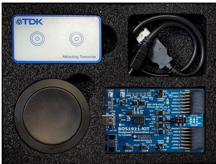
Picture 1: The PowerHap Starter Kit with Boreas 1921 Driver board inside its packaging box
