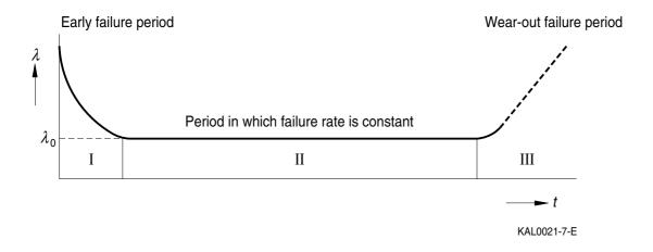
Unless otherwise specified, the given failure rate refers to the service period (phase II). During phase II, an approximately constant failure rate  $\lambda_0$  can be assumed.
