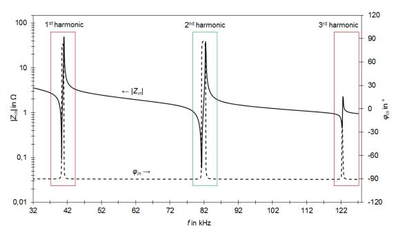
Figure 2: Typical input impedance at open-circuit output (V<sub>in</sub> = 0.1 V, no plasma).
