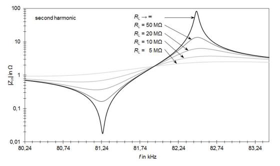
Figure 4: Simulated input impedance for different loads RL.
