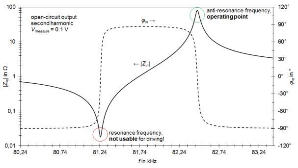
**Figure 3:** Typical input impedance around 2<sup>nd</sup> harmonic at open-circuit output (V<sub>in</sub> = 0.1 V, no plasma).
