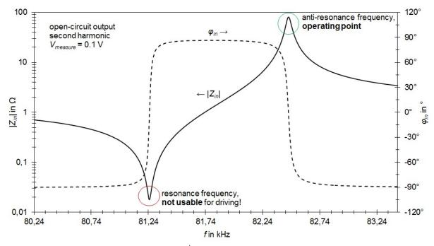
Fig. 2. Typical input impedance around  $2^{nd}$  harmonic at open-circuit output ( $V_{in} = 0.1 \text{ V}$ , no plasma).
