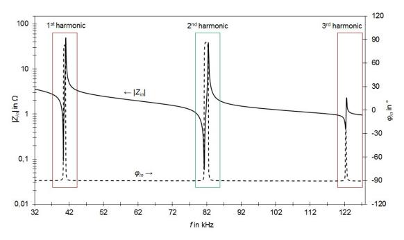
**Fig. 1.** Typical input impedance at open-circuit output ( $V_{in} = 0.1 \text{ V}$ , no plasma).
