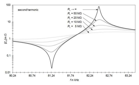
Fig. 3. Simulated input impedance for different loads R<sub>L</sub>.
