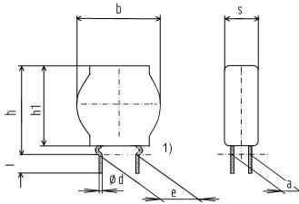
$b_{\text{max}}$ 17.5 27.0  $h_{\text{max}}$ 22.0  $h1_{max}$ = 8.7 =  $\mathbf{S}_{\text{max}}$ 7.5 ±1.0 е 2.0 (typical)  $3.5 \pm 0.5$ L =  $\emptyset d$ 0.8 ±0.05
