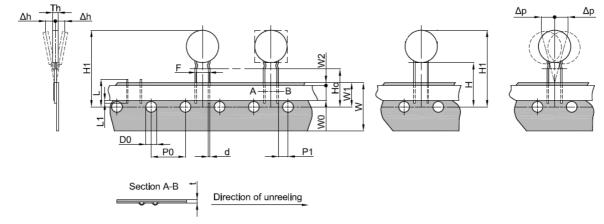
Dimensions and tolerances (taping in accordance with IEC 60286-2):
