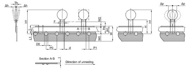
Dimensions and tolerances (taping in accordance with IEC 60286-2):
