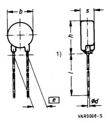
23.5  $b_{\text{max}}$ 29.0  $h_{max}$ = 9.5  $\textbf{S}_{\text{max}}$ = 10.0 ±1.0 е = 25.0 =  $I_{min}$  $\emptyset d$ 1.0 ±0.05
