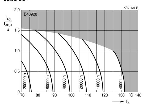
Depending on ambient temperature T<sub>A</sub> under ripple current operating condition at V<sub>R</sub> – refer to chapter "General technical information, 5 Useful life" on how to interpret useful life.
