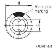
The series B41897 and B41898 have no sleeve nor minus pole marking, the positive pole is marked on the aluminum case side instead.
