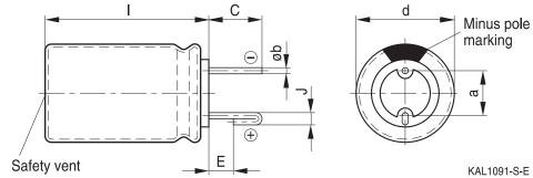
The series B41897 and B41898 have no sleeve nor minus pole marking, the positive pole is marked on the aluminum case side instead.
