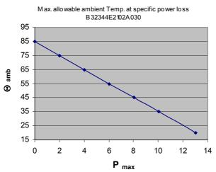
M ax. allo wable ambient Temp. at specific current (rms) B 32344E2102A 030
