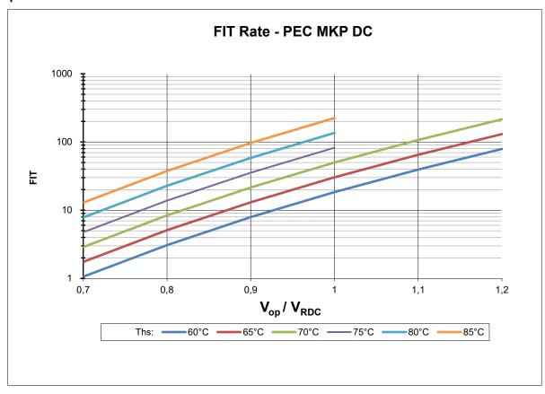
Expected Fit rate at different hot spot temperatures (Ths) and voltage VRDC
