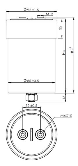
M12 stud on bottom of the aluminum case, nut (DIN 934) and toothed lock washer (DIN 6797) for fixing are standard for all types.
