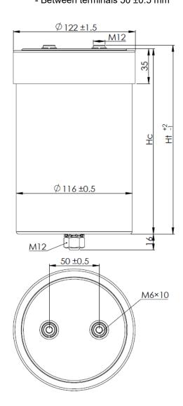
M12 stud on bottom of the aluminum case, nut (DIN 934) and toothed lock washer (DIN 6797) for fixing are standard for all types.
