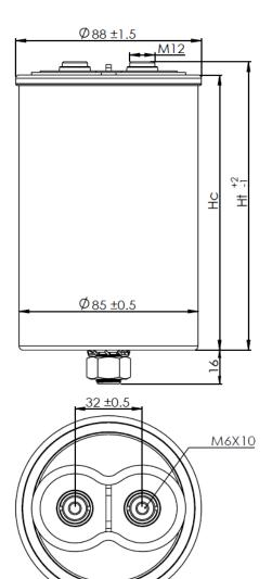
Figure 2: - B25680C - Ø 85 mm - Female terminals (M6)
