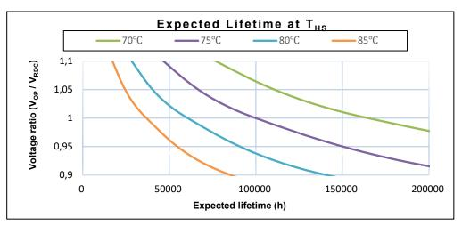
Service life t<sub>LD</sub> in hours at different hotspot temperature (T<sub>hs</sub>) and voltage V<sub>RDC</sub> for ØD≤116 mm and V<sub>RDC</sub> ≤ 2000V
