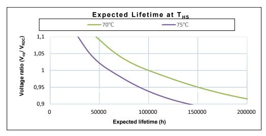
Service life t<sub>LD</sub> in hours at different hotspot temperature (T<sub>hs</sub>) and voltage V<sub>RDC</sub> for ØD=136 mm or V<sub>RDC</sub> > 2000 V
