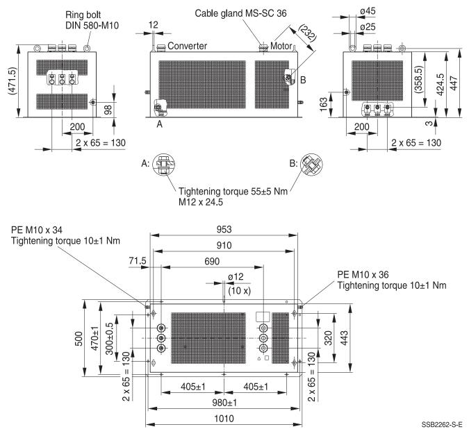
General tolerances according to ISO 2768-cL Dimensions in mm Busbar connection see section "Mechanical properties"
