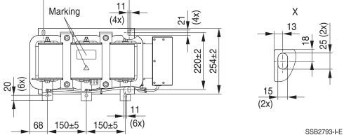
General tolerances according to ISO 2768-cL Dimensions in mm Busbar connection see section "Mechanical properties"
