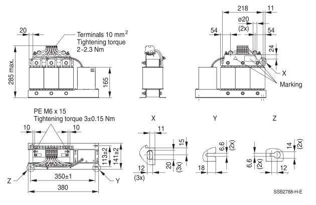
General tolerances according to ISO 2768-cL Dimensions in mm
