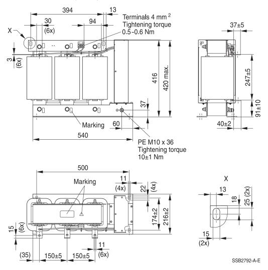
General tolerances according to ISO 2768-cL Dimensions in mm Busbar connection see section "Mechanical properties"
