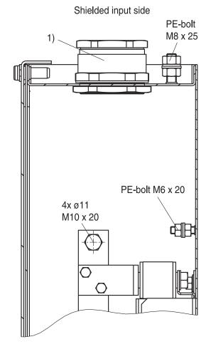
$<sup>^{1)}</sup>$  Cable glands PG 42\* with indented sealing ring, for cable diameters [mm]: 29 ... 31 / 32 ... 34 / 35 ... 37 / 38 ... 40
