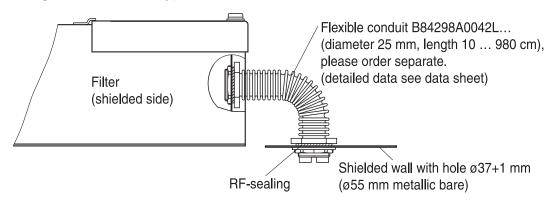
Note: The bending radius of the flexible conduit depends on the used type of cable
