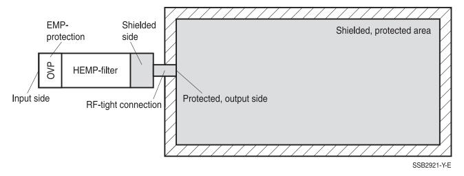
Filters B84299D2320E303, B84299D1101E303 for assembly at outside to the shielded wall
