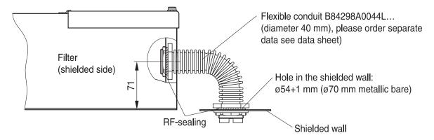
Note: The bending radius of the flexible conduit depends on the used type of cable
