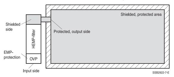
Filters B84299C2320E313, B84299C1101E313 for assembly at inside to the shielded wall
