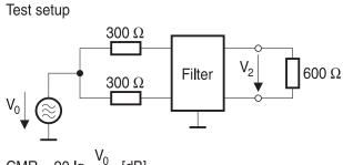
CMR = 20 lg  $\frac{V_0}{2 V_2}$  [dB]
