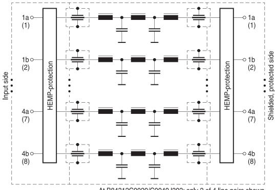
At B84312C0020/C0040J303: only 2 of 4 line pairs shown At B84312C0030J303: only 4 of 8 lines shown
