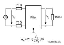
Symmetrical measurement circuit with  $Z_L=150\;\Omega$
