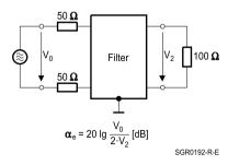
Symmetrical measurement circuit with  $Z_{L}=100\;\Omega$
