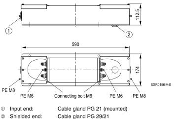
(cable gland PG 29, PG 21 and reducer ring in accessory bag)
