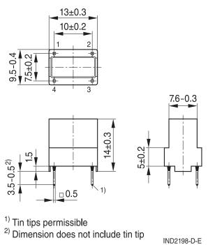
Tolerances to ISO 2768-c / ISO 8015. Size ISO 14405 E All dimensions in mm
