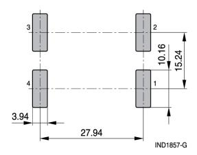
Part tolerances to ISO 2768-cL / ISO 8015. Size ISO 14405 (E) All dimensions in mm
