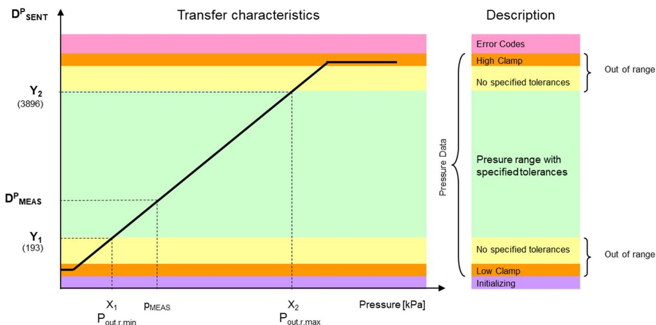
Conversion SENT's Pressure Data to physical pressure acc. to conversion formula below.
