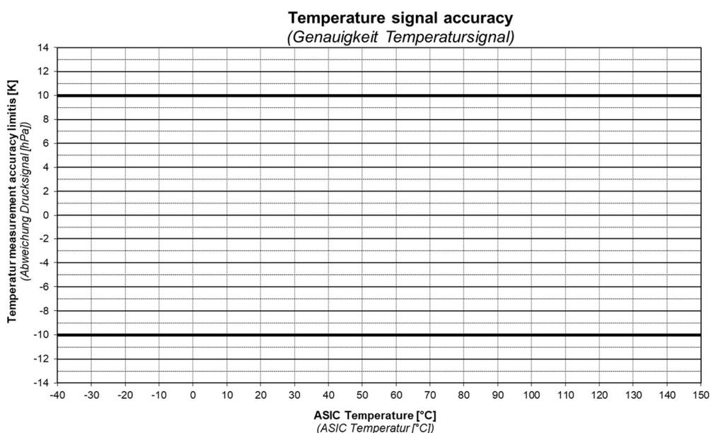
ASIC temperature measurement accuracy: +/- 10 K
