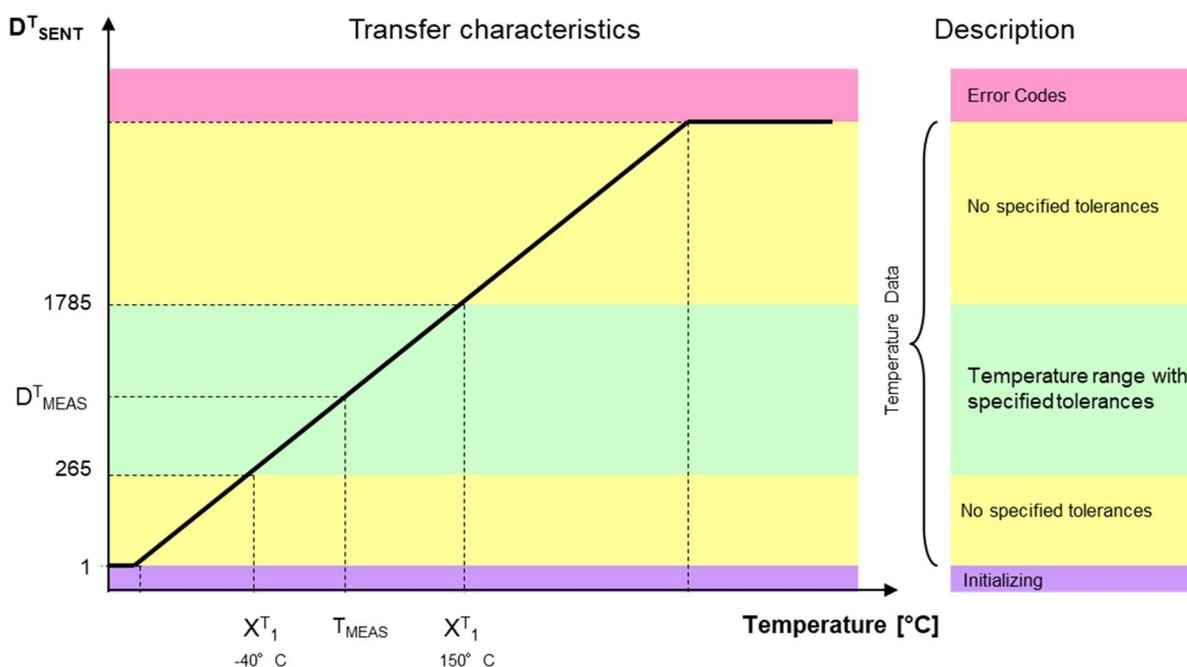
Conversion SENT's Temperature Data to physical Temperature acc. to conversion formula below.
