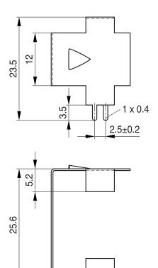
Dimensional tolerances +/-0,2 Dimensions in mm
