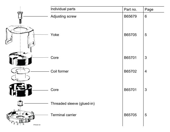
Example of an assembly set for printed circuit boards
