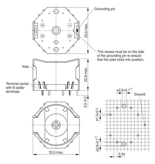
1) The 2.8 mm hole is only necessary for additional fixing with M2.5 screw.
