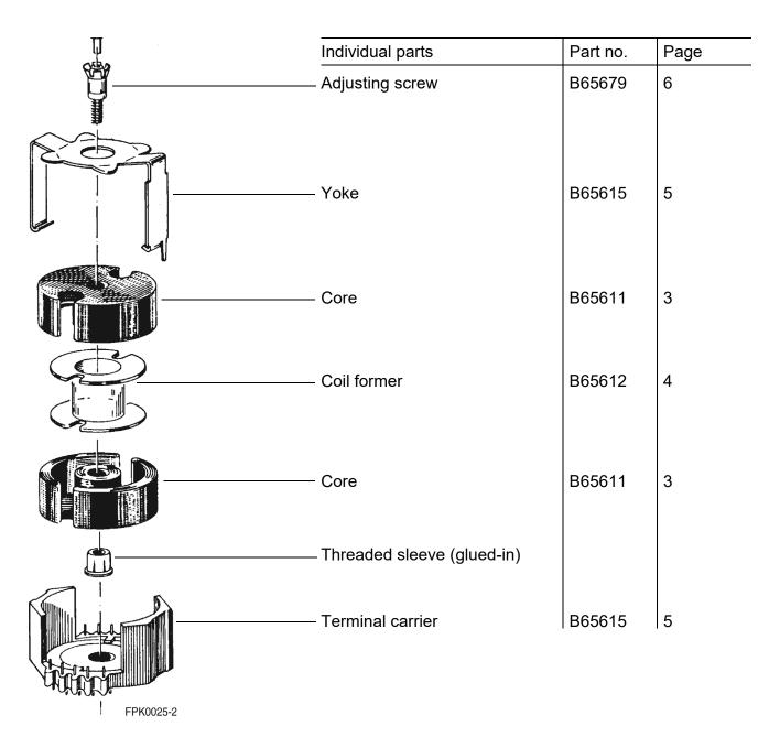
Example of an assembly set for printed circuit boards
